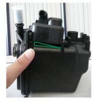
1 Put the fuel heater into the guide in an oblique position.
