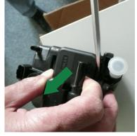
1 Press up the plastic bracket with the help of a screwdriver and pull out the fuel heater at the same time.
