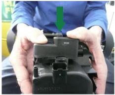
**3** Push the fuel heater down by using both thumbs until you hear a click sound.
