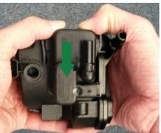
**2** Push the fuel heater up to the stop.
