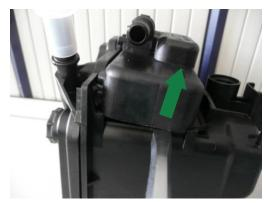
**2** Use the screwdriver to lever the heater out.
